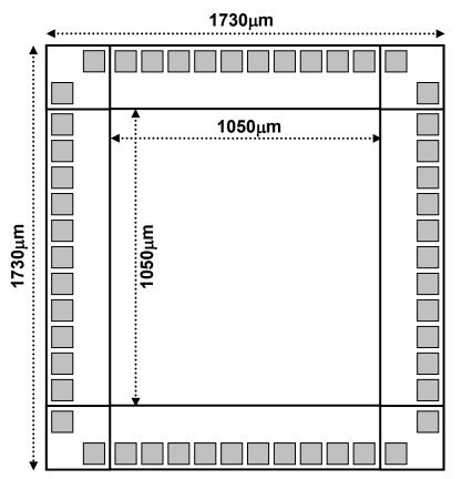
Figure 3. Schematic picture of a  $3 \text{mm}^2$  chip with 40 generic pads four  $V_{DD}$  and four  $V_{SS}$  pads (total 48 pads), which will be shared between a number of projects.
