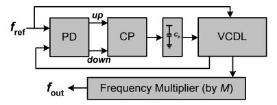
Figure 1: System Block diagram of DLL-based frequency multiplier.
