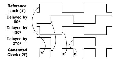
Figure 2: Example of timing for a frequency multiplier
