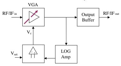
Figure 1: Block diagram of AGC using VGA and log amplifier detector.
