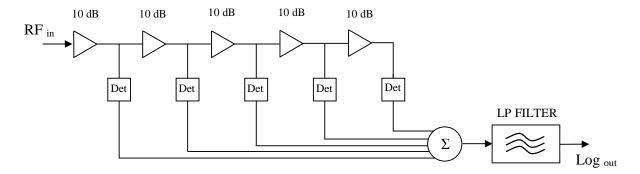
Figure 2: Block diagram of Log Amplifier detector.
