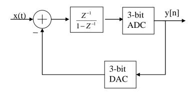
Figure 1: First-order Sigma-Delta modulator architecture.
