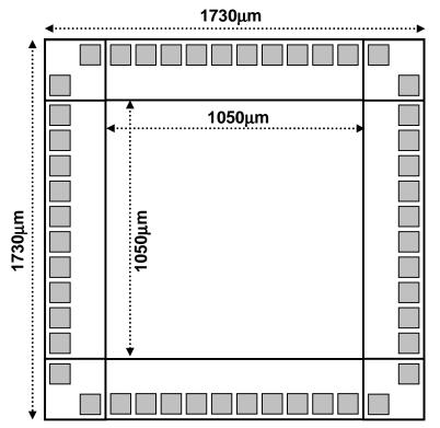
Figure 2: Schematic picture of a  $3 \text{mm}^2$  chip with 40 generic pads four  $V_{DD}$  and four  $V_{SS}$  pads (total 48 pads), which will be shared between a number of projects.
