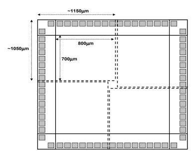
**Fig 3:** A 5mm<sup>2</sup> chip will be shared by 4 independent projects (4 teams). Each project will utilize a  $700x800\mu m^2$  area for core layout and 17 pads.
