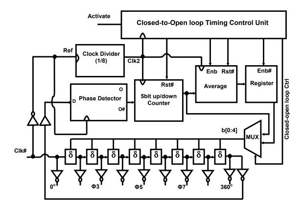
Fig.1: Organization of the multiphase clock generator
