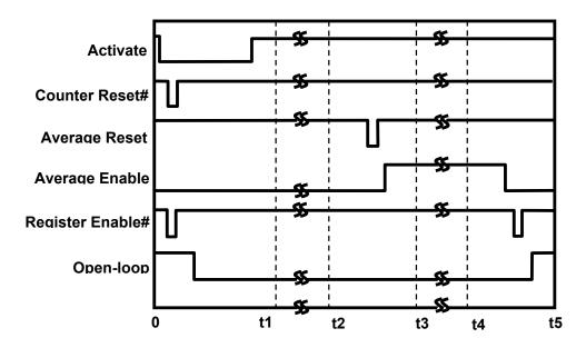
Fig.2: Timing diagram of the closed-to-open loop control unit.
