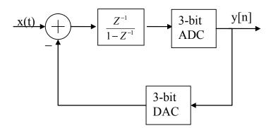
Figure 1: First-order Sigma-Delta modulator architecture.
