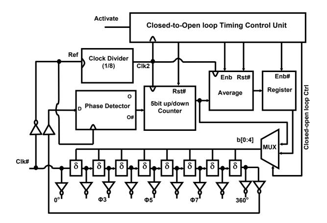
Fig.1: Organization of the multiphase clock generator
