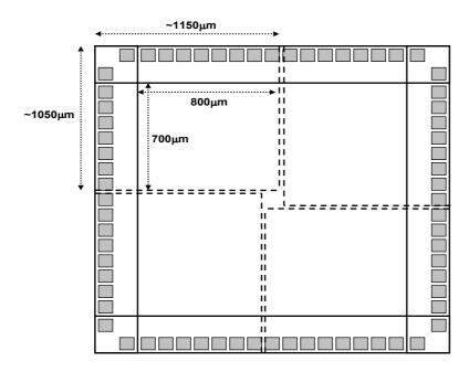
**Fig 3:** A  $5mm^2$  chip will be shared by 4 independent projects (4 teams). Each project will utilize a  $700x800\mu m^2$  area for core layout and 17 pads.
