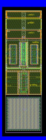
AUPRIOP (not yet available) – Analog Input/Output PAD - No ESD protection - Signal accessed in metal 2 on core-side of the PAD Suitable for high-speed I/O and power supply with different voltage than core
