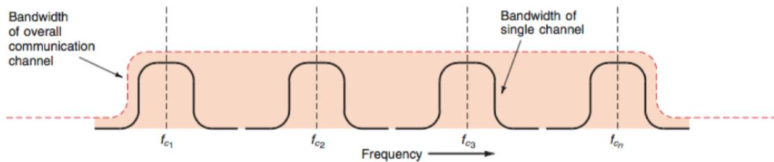
**Figure 10-4** The receiving end of an FDM system.
