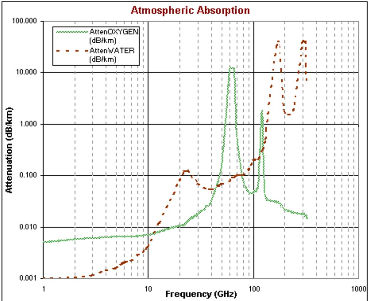
Electromagnetic waves are absorbed in the atmosphere according to wavelength. Two compounds are responsible for the majority of signal absorption: oxygen ( $O_2$ ) and water vapor ( $H_2O$ ). The actual amount of water vapor and oxygen in the atmosphere normally declines with an increase in altitude because of the decrease in pressure, so these graphs apply from sea level to around 1 km altitude.
