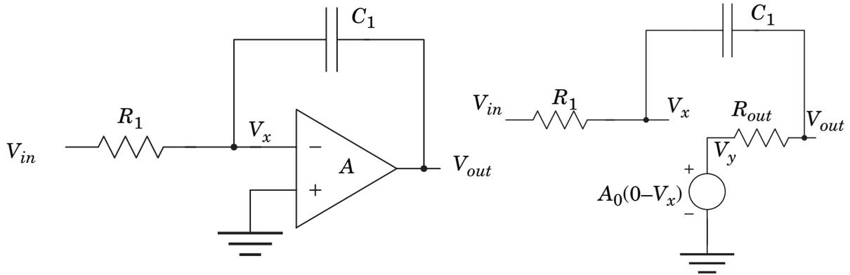
**Figure 3.1** A Miller integrator. a) Amplifier description, b) Macro model description.
