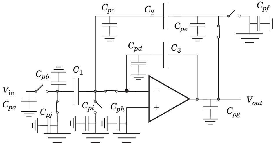
**Figure 4.1** The SC circuit with capacitive parasitics due to the capacitor and the switches.
