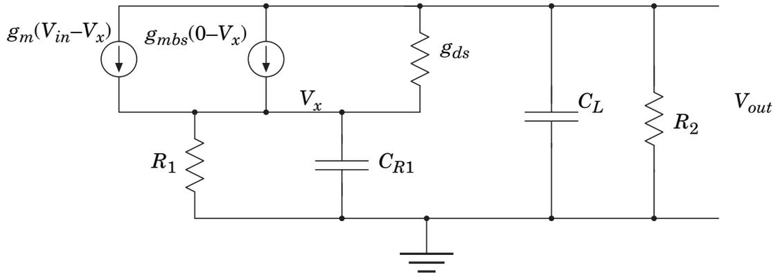
**Figure 2.1** The small-signal model of the source-degenerated common-source amplifier.
