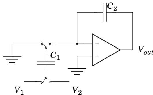
**Figure 4.1** A switched-capacitor circuit in clock phase 1.
