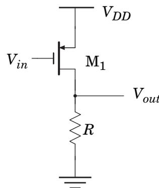
**Figure 1.1** A simple amplifier structure with resistive load.
