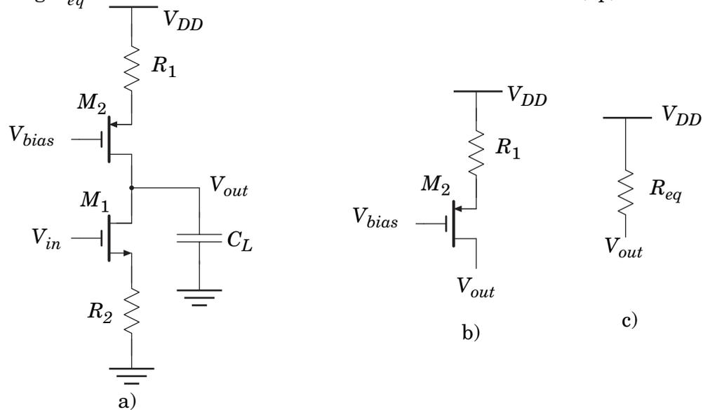
**Figure 2.1** An amplifier. a) The whole amplifier. b) The PMOS and resistor part. c) The equivalent small-signal circuit of b).
