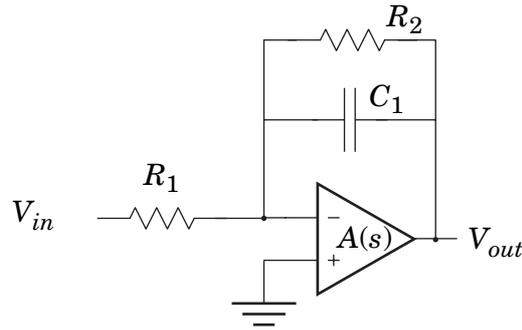
**Figure 3.1** An active-RC circuit.
