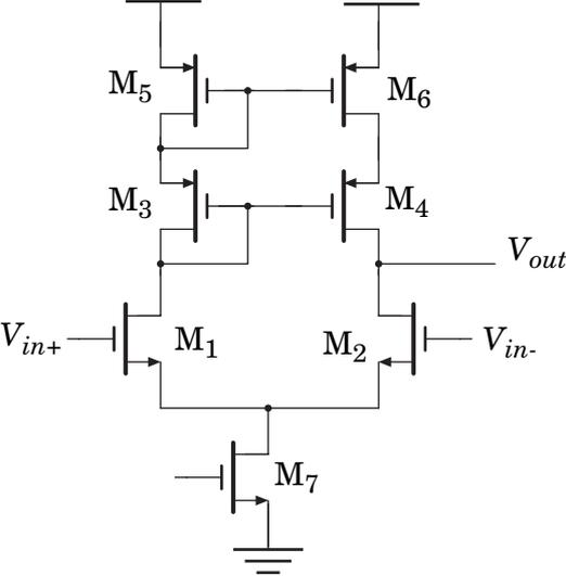
**Figure 5.1** A CMOS amplifier circuit.
