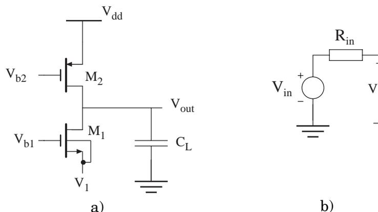
**Figure 1.1** a) A CMOS gain stage. b) Input voltage source.
