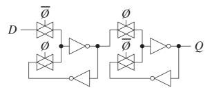
b) During rise and fall times, all transmission gates in the flip-flop will conduct (weaker than normal). If the rise or fall time are longer than the propagation time of the weakly conducting path, the flip-flop becomes transparent and will fail to store the signal properly.
