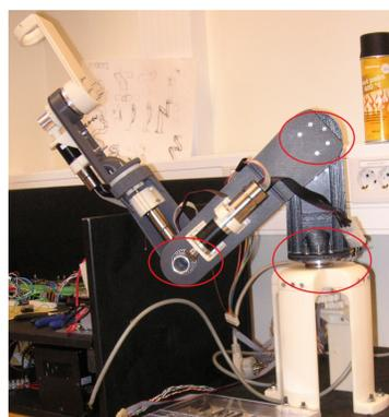
which in turn is connected to the computer. The robot has 3 degrees of freedom and a range of approximately 1 meter in all directions.
