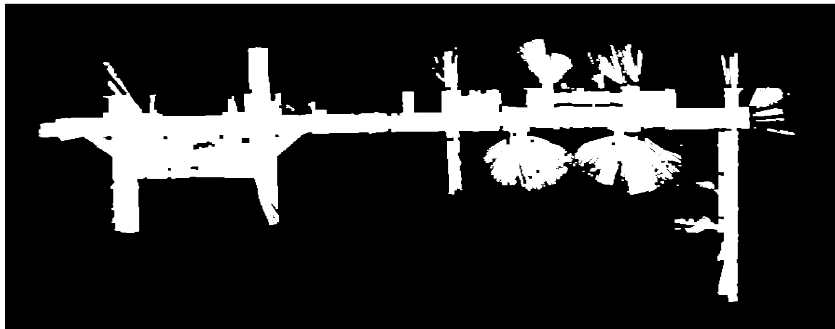
Figure 22: A binary version of the occupancy gridmap is used in the pathfinding algorithm.
