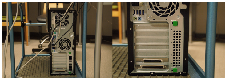
Figure 8: The computer back panel with A/D and D/A slots. [6, Fig. 2]
