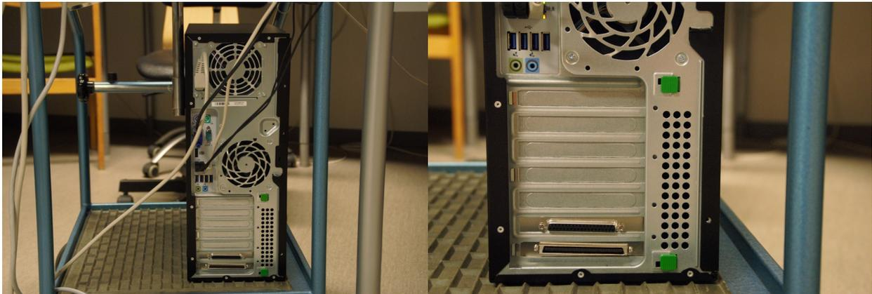
Figure 2: The computer back panel with A/D and D/A slots.
