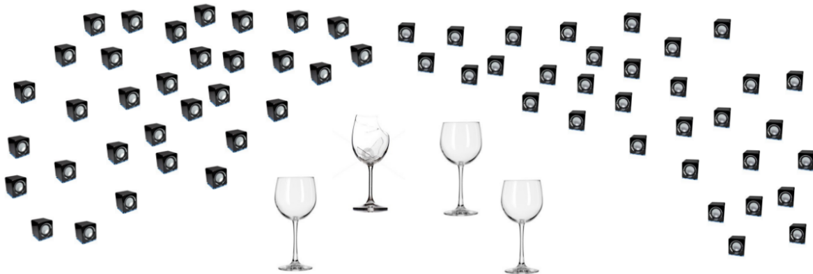
Figure 1. A possible setup for a demonstration of massive MIMO beamforming.
