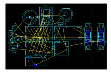
The figure below shows the ratsnests connecting pads in a design.
