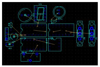
• Use **Part Shoving** to move one part and have Ultiboard automatically push other parts on the board out of the way to create enough available space for the part.
