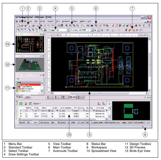
Ultiboard is the PCB layout application of National Instruments Circuit Design Suite, a suite of EDA (Electronics Design Automation) tools that assists you in carrying out the major steps in the circuit design flow.
