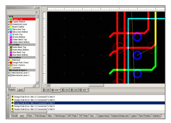
Although the design rules and netlist check runs automatically, you may want to run a final check of the board's integrity prior to saving or exporting the design.
