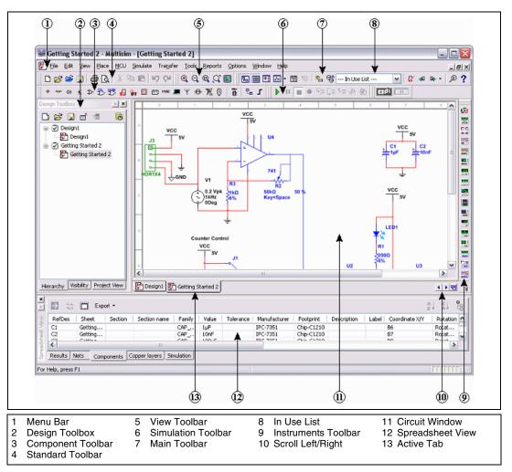
Multisim is the schematic capture and simulation application of National Instruments Circuit Design Suite, a suite of EDA (Electronics Design Automation) tools that assists you in carrying out the major steps in the circuit design flow. Multisim is designed for schematic entry, simulation, and feeding to downstage steps, such as PCB layout.
