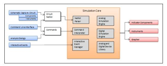
A simulation in Multisim runs in one of two simulation modes: Interactive Simulation Mode or Analysis Simulation Mode.
