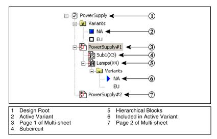
The **Project View** tab is where you can see the files assigned to a project. A project is a collection of files. For example, all the circuit files making up a design may be grouped together in a project, as well as external design documentation, simulation output, reports, and PCB layouts generated with Ultiboard.
