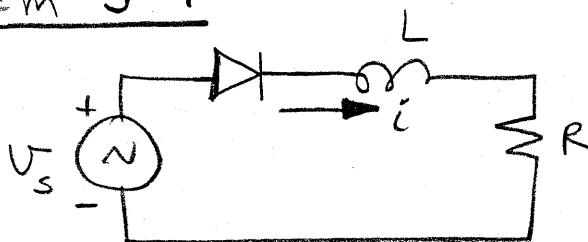
$$V_s = 120 \text{ V at } 60 \text{ Hz}$$
