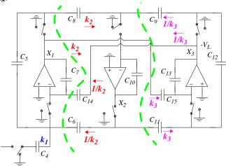
Scale the filter so that the relation between the OPamp outputs and the input signal is unity  $(L_{\infty}\text{-norm})$ . We are scaling the filter to keep the signal levels at wanted levels. The principle of scaling can be described by dividing the net into subnets. The subnets have a number of inputs and outputs. If the inputs are scaled with a constant  $k_i$  all nodes of the subnet will be scaled with a factor  $k_i$ , as well as we have to scale all outputs with  $1/k_i$ .
