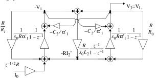
The two integrators (inverting amplifiers with and without delay) are replaced with their corresponding SC circuits.
