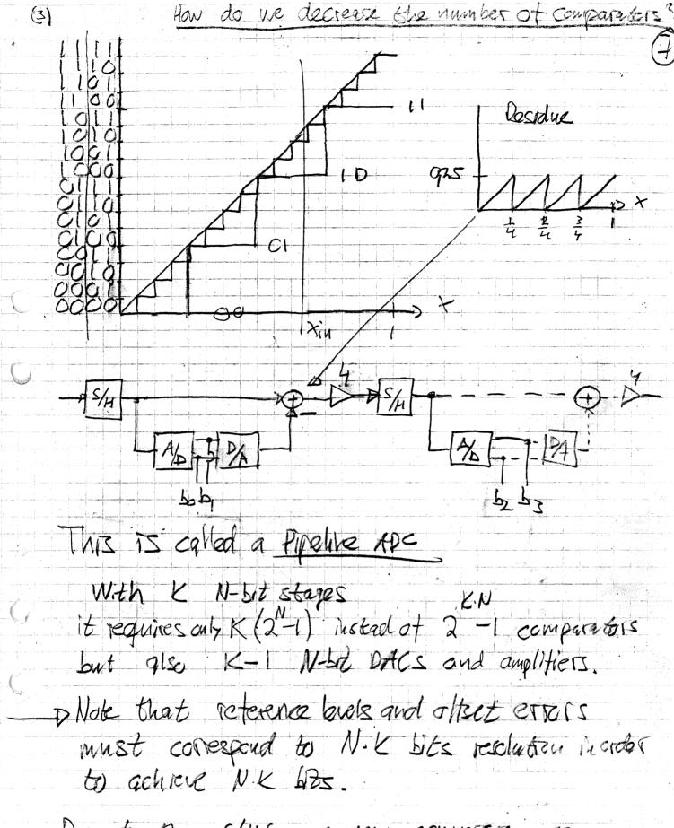
Due to the SHI'S, a new conversion can start as soon as the MSBS are converted. The output bits are then stored in shift regretors
