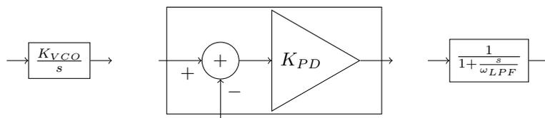
Figure 6: Linear models for Voltage Controlled Oscillator, Phase Detector, and Low-Pass Filter.
