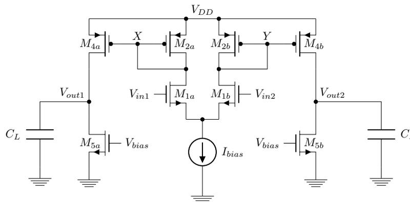
Figure 2: A fully differential amplifier.
