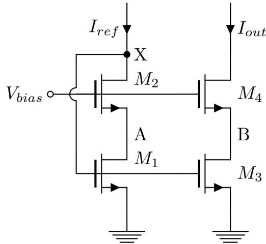
Figure 3: A low-voltage cascode current mirror.
