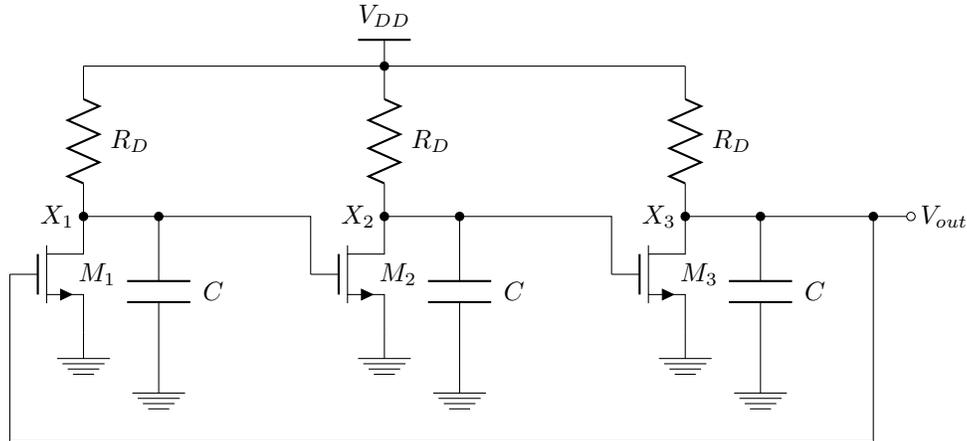
Figure 5: 3-stage ring oscillator
