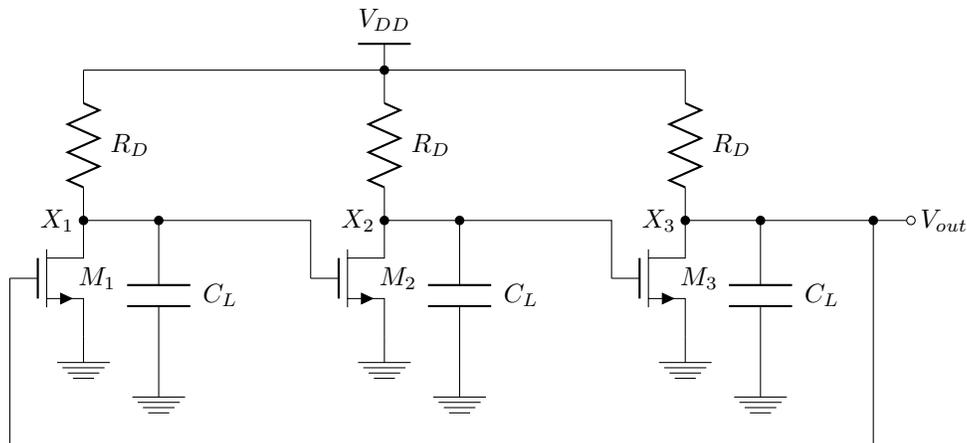
Figure 5: 3-stage ring oscillator
