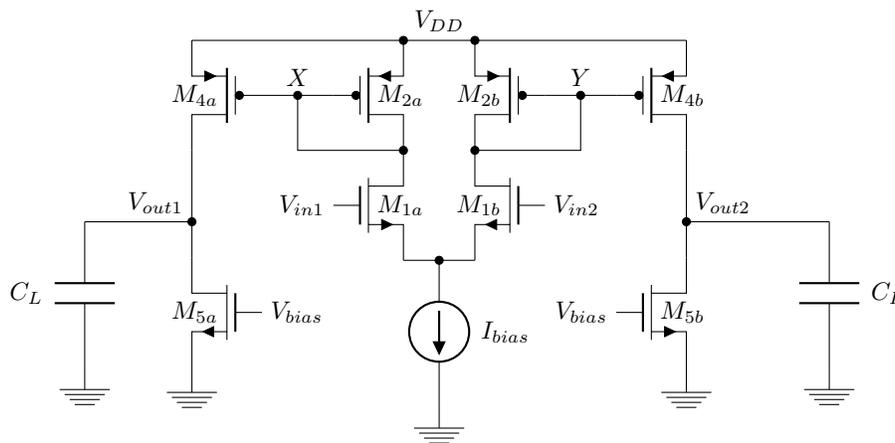
Figure 2: A fully differential amplifier.
