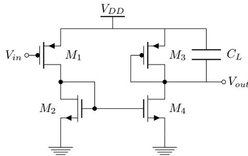
Figure 1: Schematic of a single-ended amplifier.
