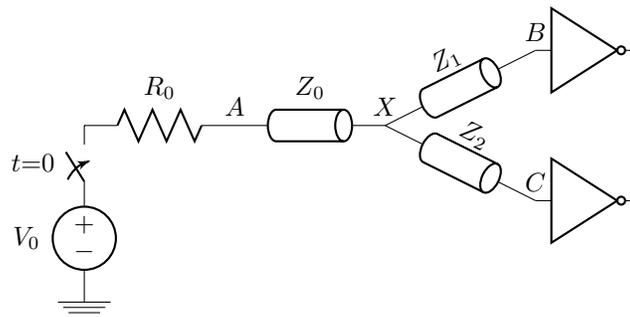
Figure 4: Transmission line circuit.
