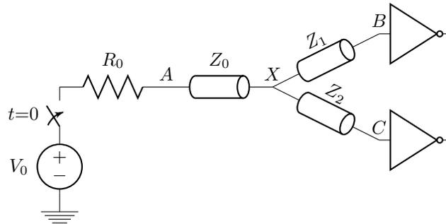
Figure 4: Transmission line circuit.
