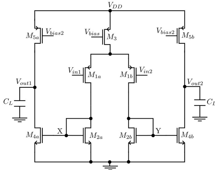
Figure 2: A fully differential amplifier.
