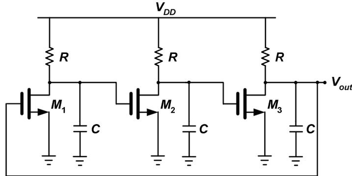
Fig. 4. A three-stage ring oscillator.
