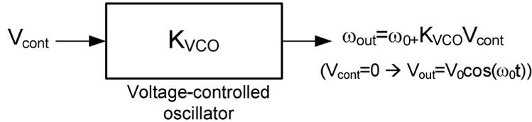
Fig. 4. A voltage-controlled oscillator.
