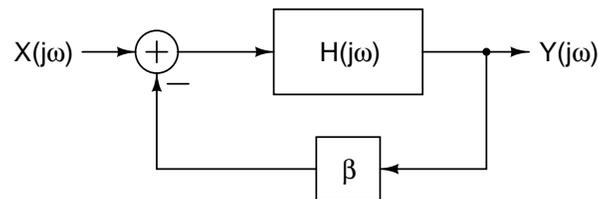
The closed-loop transfer function of this system can be found to be
