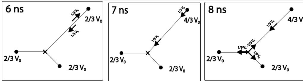
at 7.5ns:  $V_A = 2/3V_0$ ,  $V_B = 4/3V_0$  and  $V_C = 2/3V_0$
