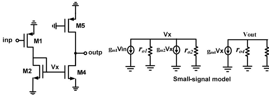
Writing two KCLs at nodes  $V_x$  and  $V_{out}$  and noting that  $g_{ds} = r_o^{-1}$  we get:
