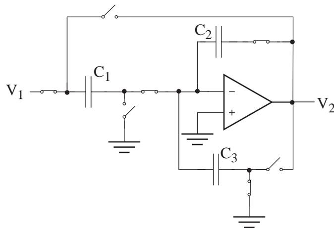
**Figure 4.1** A switched capacitor circuit
