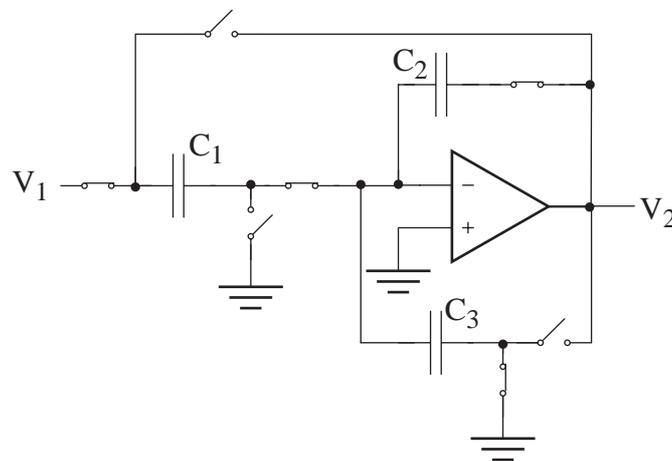
**Figure 4.1** A switched capacitor circuit
