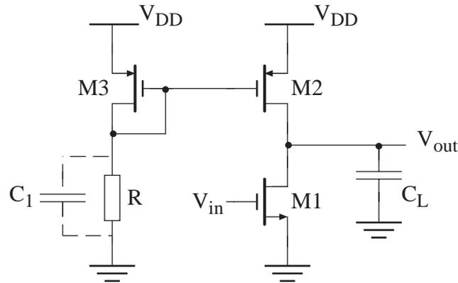
**Figure 3.2** A noisy common source gain stage
