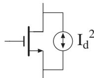
**Figure 3.1** Thermal noise model for a MOS transistor
