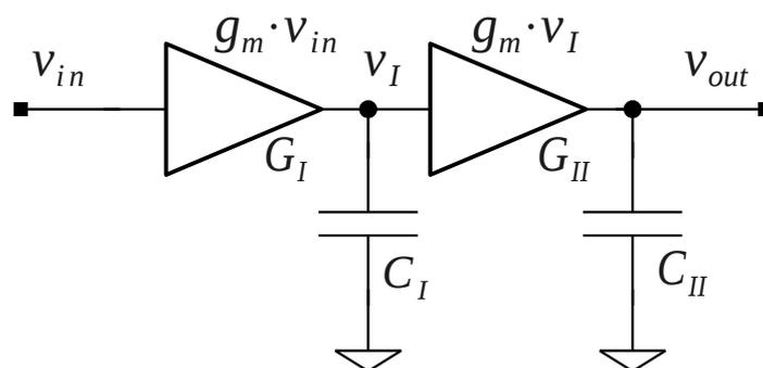
Figure 3.1: A two-stage amplifier.
