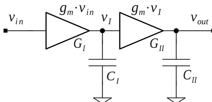
Figure 3.1: A two-stage amplifier.
