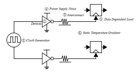
Figure 0.2 Sources of Skew and Jitter in Clock Distribution.
